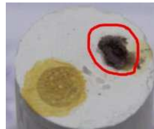
Figure 17 - iodine test on a piece of spent grain from experiment 33 (0.95 mm) (circled in red)
